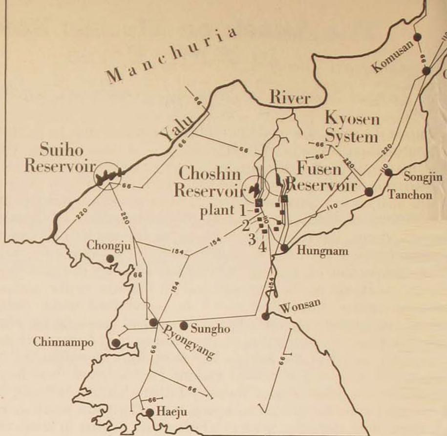
The hydro-electric power plants and main interconnecting transmission lines. Town names locate strategic industrial targets, showing their proximity to power network.
